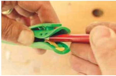
▲ The 'Classic' carpenter's pencil is held firmly in the holder with a spring clip
